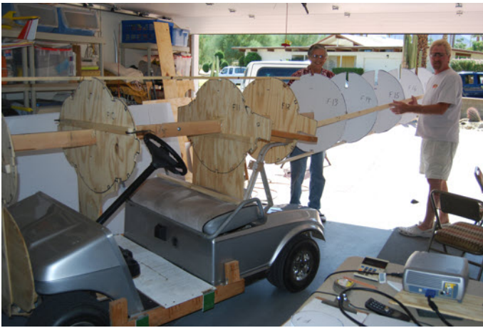
Photo 1, Truss frame and formers on cart.
